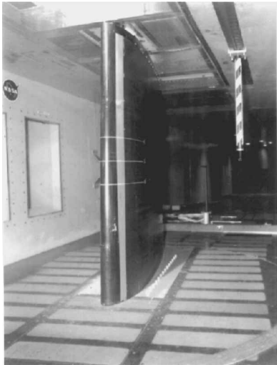
Fig. 2 Model installed in IRT.
